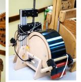
His next jig was a *guitar side bender*. This shop-built jig is made of plywood with a removable inner form that is used to provide the desired bends in the side piece. The outer shell of the jig is also plywood and is fitted with 3 lamp-holders in the bottom and a top bridge piece which held the clamping screw that is used to force the inside bend into the side piece on the form. The bulb wattages are determined by trial and error and Bernd noted this could get
