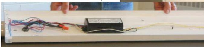
he reconfigured his fixture by showing us how to remove the ballast and rewire it to use end-fed LED retrofit tubes. Great job Tony! Thanks.
