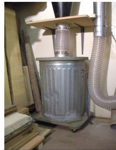
Chip collection bin on rolling base connected to chip outlet of the SDD
