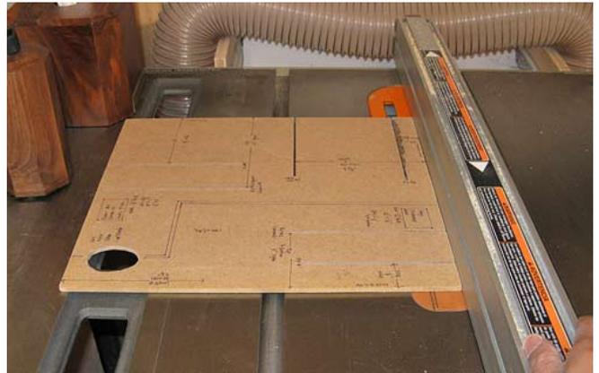
**Machinery and Tool Mistakes:** Using a machine that's not properly set up can create and compound mistakes. When a rip fence is not parallel to the blade, for example, the mistakes are usually not apparent until you are at the late assembly stage. At this point, a quick fix will be almost impossible as all the mating pieces have been cut. You can prevent most of these unnecessary slips by performing regular tune-ups and using scraps to test the critical set-ups or cuts.
